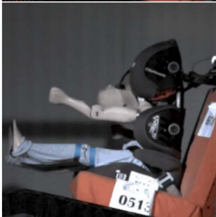
Fig. 10. Video frames comparing the overall motion of the ATD head and torso at the point of maximum forward head excursion for one representative test of each condition (right: no HSS; left: HSS).
