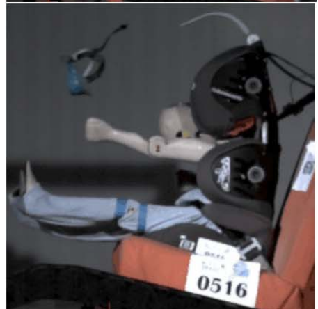
Fig. 10. Video frames comparing the overall motion of the ATD head and torso at the point of maximum forward head excursion for one representative test of each condition (right: no HSS; left: HSS).
