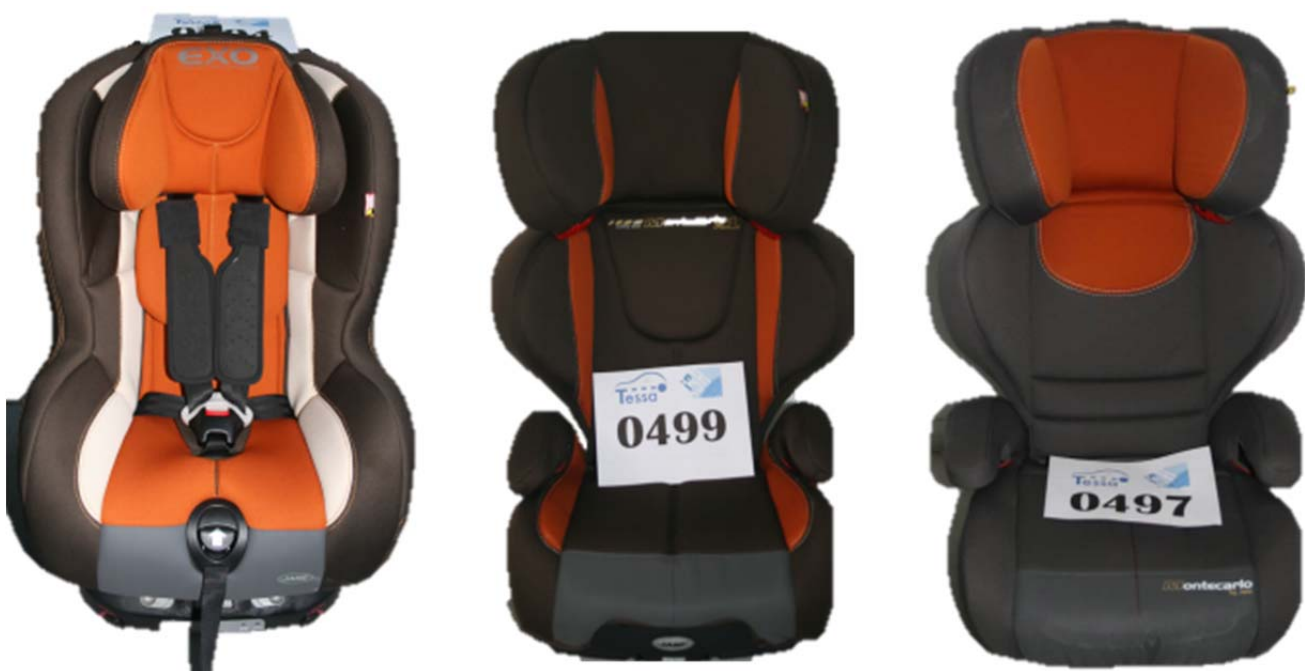
Fig. 2. The three CRS used in this study: forward facing seat (ISOFIX, top-tether), high-back booster seat (ISOFIX) and high-back booster seat without ISOFIX.
